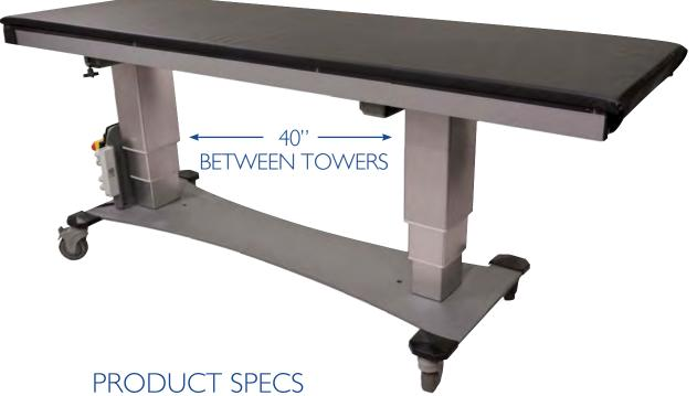
PATIENT WEIGHT CAPACITY 450lbs. (205kg.) TOP 24" (61 cm) W, 78" (198 cm) L MOTION I height range 24" - 40" (61 cm × 102 cm) MOTION 2 23" (56 cm) overall manual travel top MOTION 3 Trendelenburg tilt +/ -14° **CONTROLS** I foot, I hand TABLE WEIGHT 320lbs. (813kg.) WARRANTY 4 year REGULATORY FDA, ETL, CE
